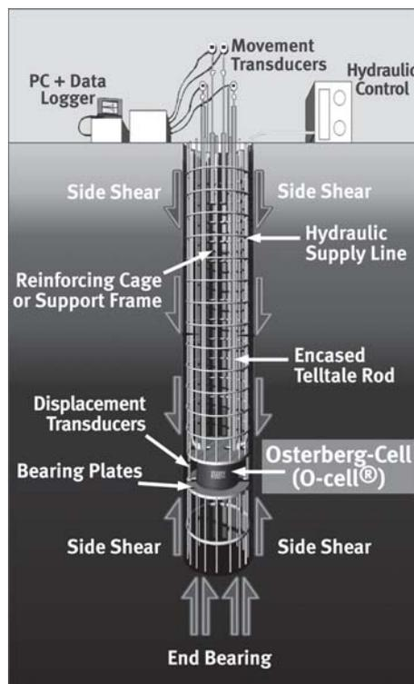
**Fig. 1** Static pile load test set-up using the Osterberg Cell method
