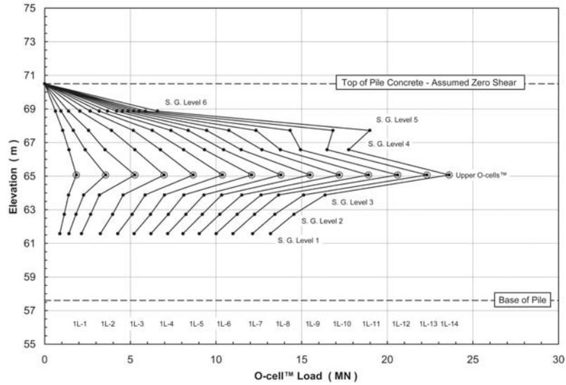
Fig. 6 Load-distribution curves – Stage 1
