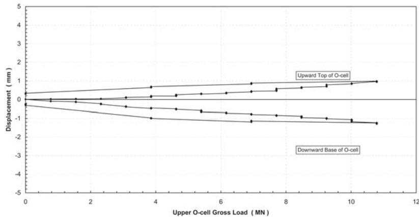
The single level array used at test pile 2 consisted of two O-cells of 3.6 MN nominal capacity each. This resulted in a total test capacity of 14,4 MN. The test mobilised a resistance of over 10 MN. The results of both tests allowed the pile design to be optimized. Permitting on one hand, advantage to be taken of the high bearing capacity of the limestone and on the other hand, that no damage would be caused to the highly valued mineral water sources.
