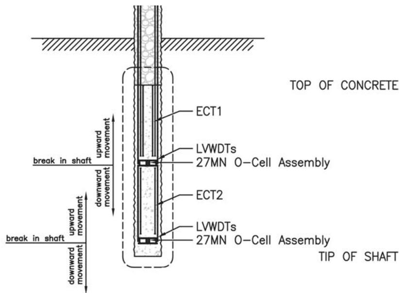
**Fig. 3** Location of multiple O-cell levels
