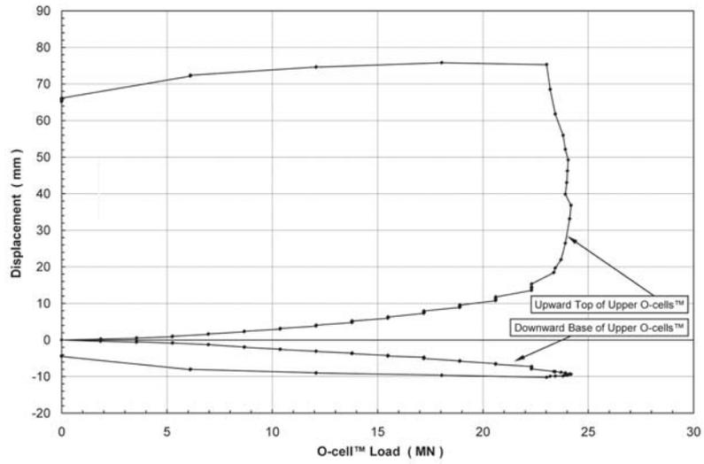
Fig. 5 Load-movement curves – Stage 1
