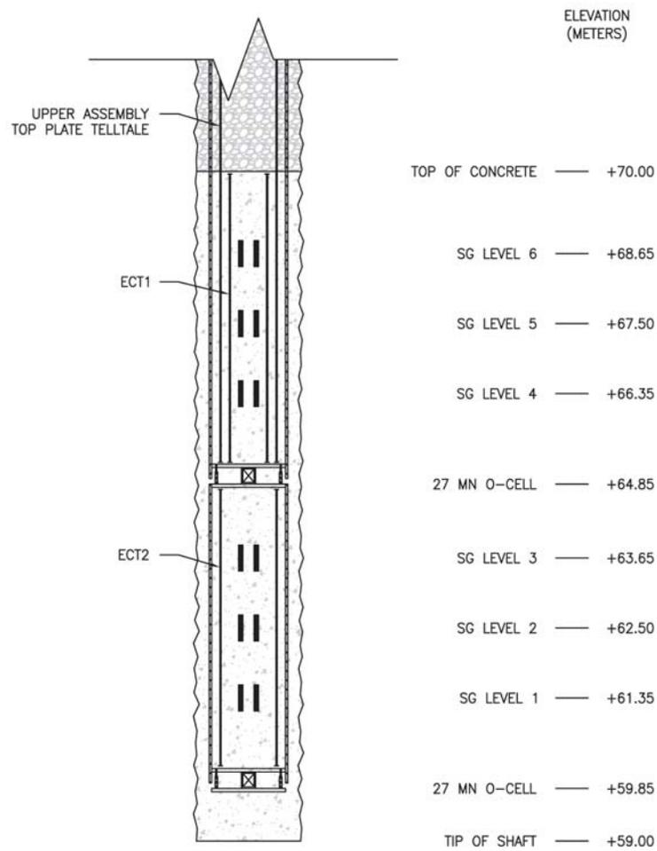
**Fig. 4** Instrumentation to determine shaft strain distribution
