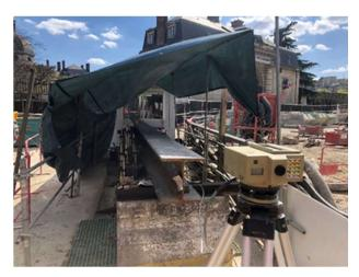
Fig. 6. Testing underway, footprint is the same as the foundation element. The beam is for datum reference only.
