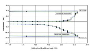
Fig. 7. Load - displacement top and base of O-cell movement.
