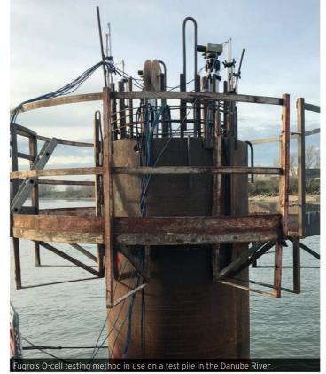
A bi-directional testing system is being used in the development of foundations for a new cablestayed bridge between Hungary and Slovakia
